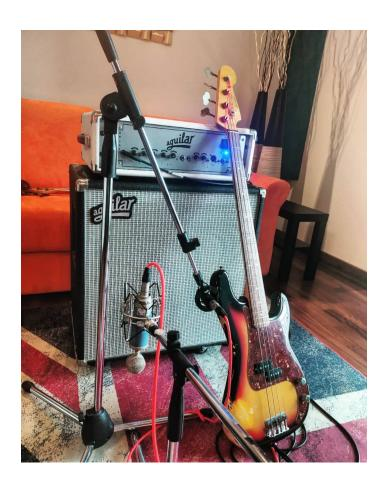
The DB 751 combines the legendary tube-driven tone of the DB 750 with greater EQ control. A perfect combination of raw power and excellent tone, the DB 751 continues the legacy set by the world famous DB® 750. Delivering 975 Watts at 2 ohms and 750 Watts at 4 ohms, this amp has the headroom you need to play any size venue
